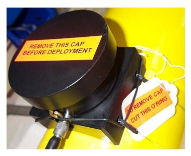
The Flntu Sensor has a protective cap that must be removed before deployment. To remove cap cut black O-ring which holds it in place.
