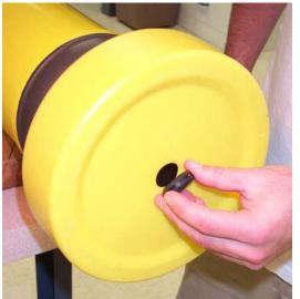
2. Carefully pry black rubber plug out of bottom center of yellow plastic cowling to verify bladder inflation (per below). **Be sure to replace plug before deployment.**
